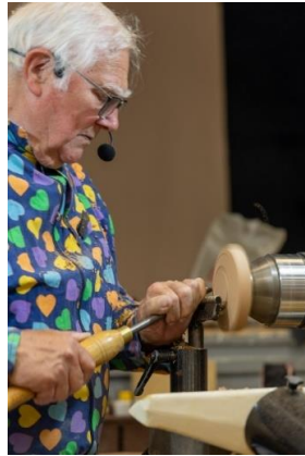
Turning the foot and the outside (3477)
